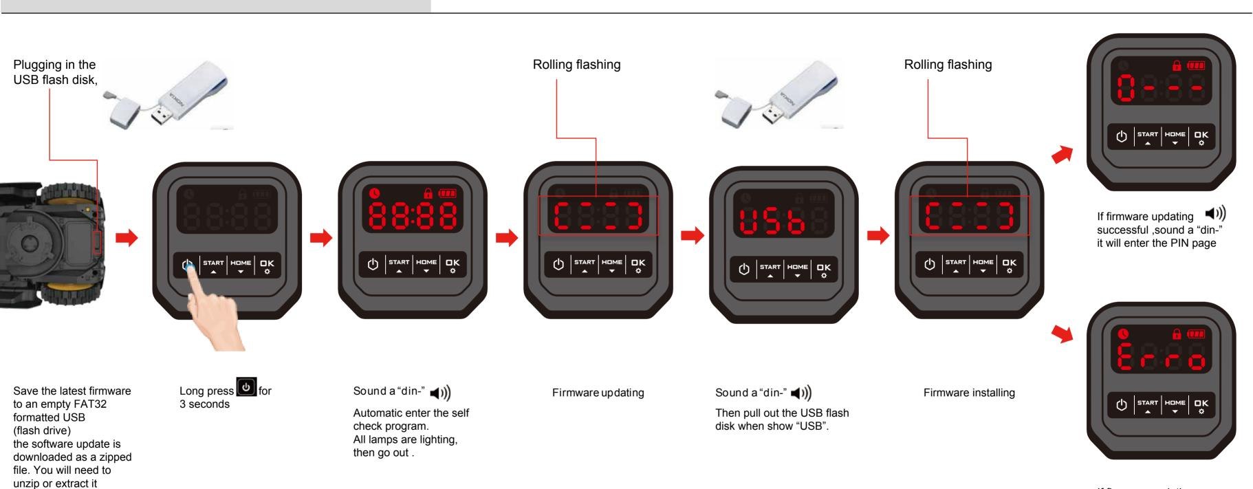
If firmware updating not successful , Show "ERRO" flashing and sound a "din-din , din-din, din-din" . Landxcape automatic () restarting with old firmware .
